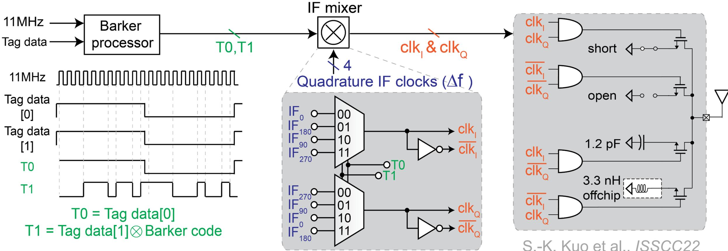
Step1: Generate Barker code modulated data with on-chip 11MHz clock
