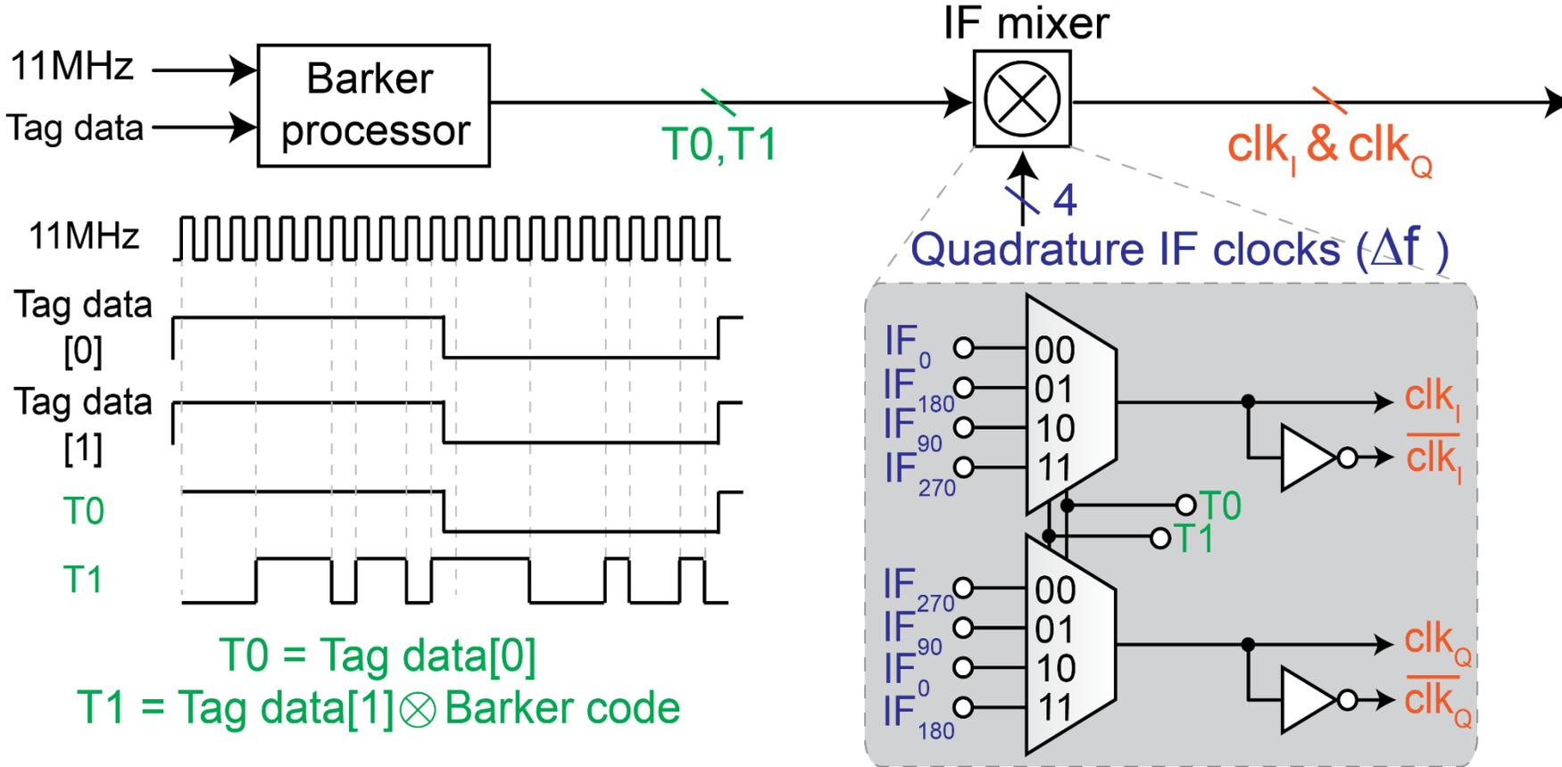
Step1: Generate Barker code modulated data with on-chip 11MHz clock
