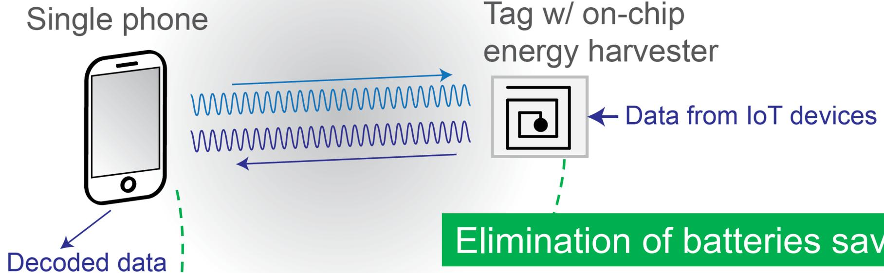
Single access point enables RFID-like operation
