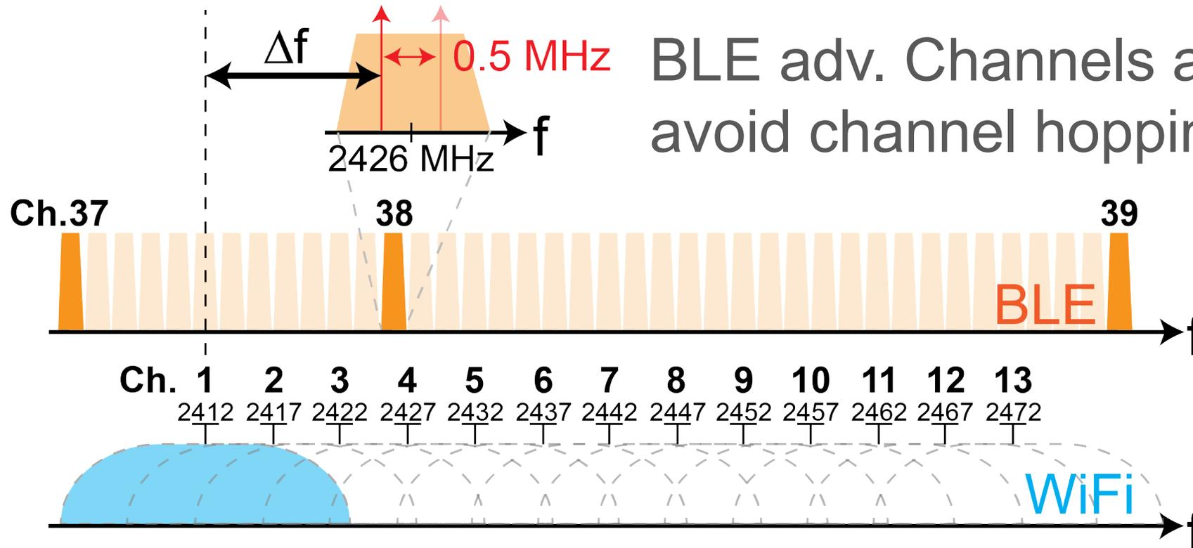
BLE adv. Channels are used to avoid channel hopping ambiguity
