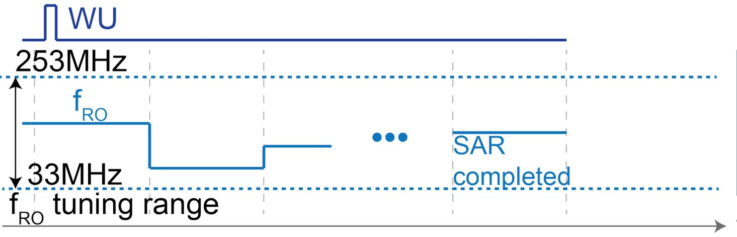
SAR FLL locks the ring osc. output to the desired freq. within 15 cycles (0.915msec)
