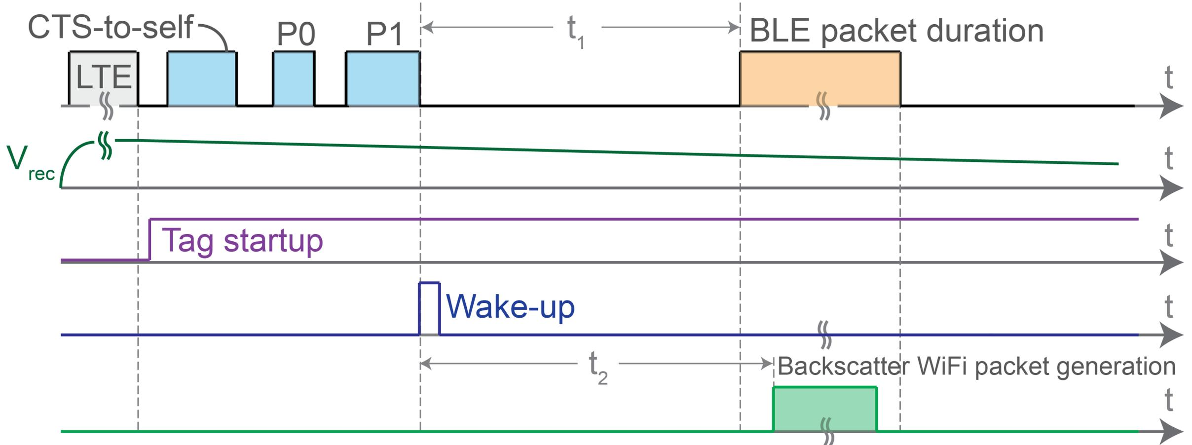
Step 3: Perform backscatter within BLE packet duration ( $t_2 > t_1$ )
