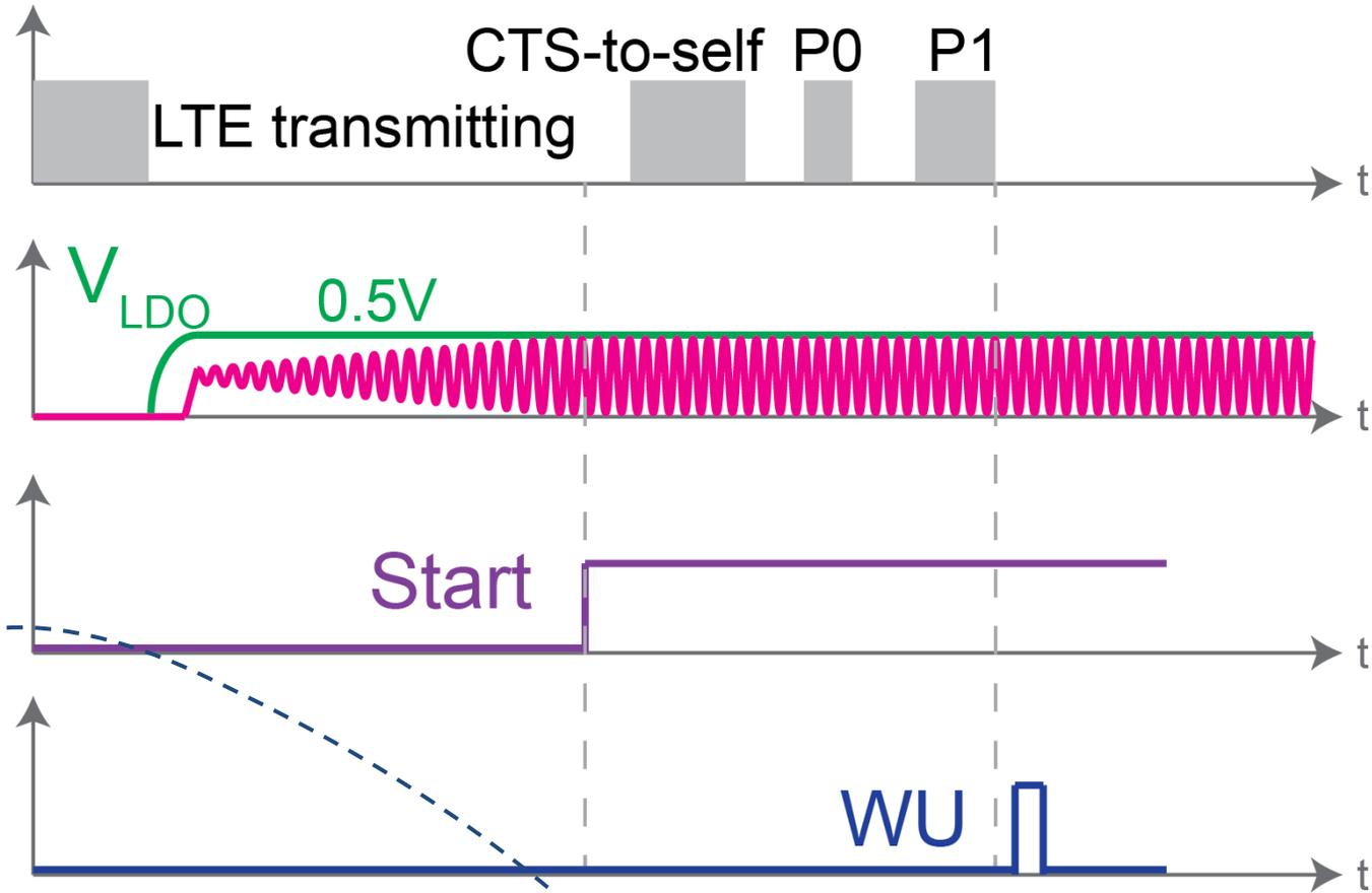
An ED and a comparator are used to determine the XTAL startup
