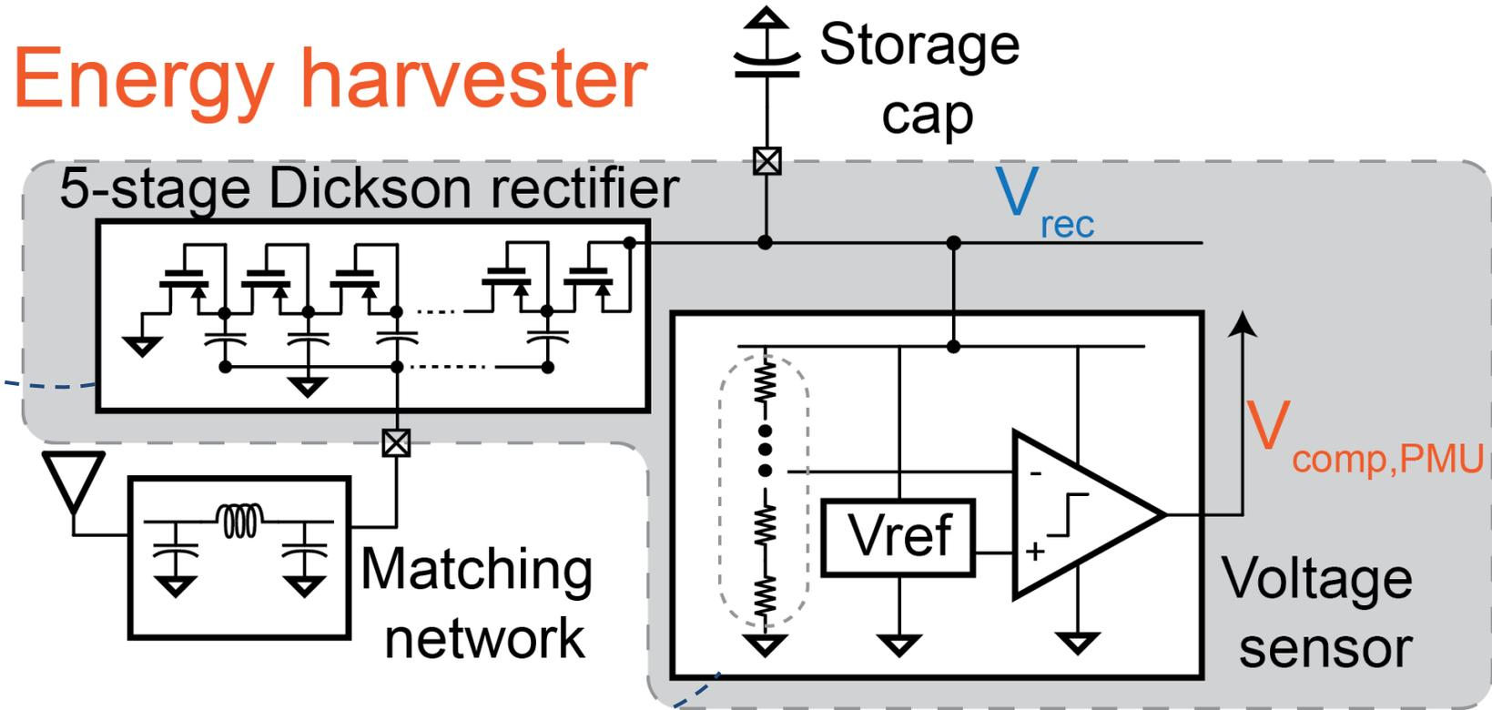
$V_{rec}$  is sensed by a voltage ref. generator, a trip voltage generator and a comparator
