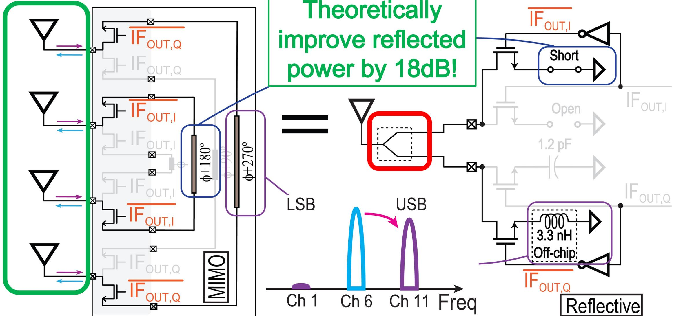
12.2: Improving the Range of WiFi Backscatter Via a Passive Retro-Reflective Single-Side-Band-Modulating MIMO Array and Non-Absorbing Termination
