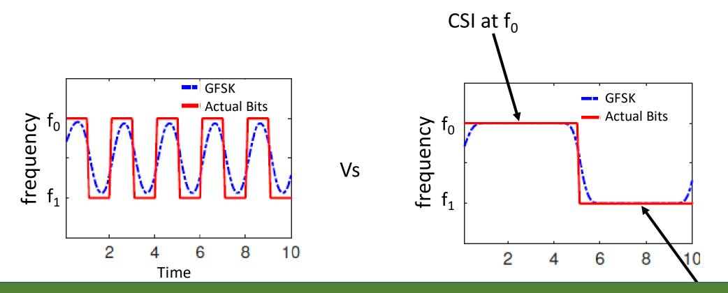
Now we can estimate CSI at  $f_c$  subcarrier as (CSI at  $f_0$ +CSI at  $f_1$ )/2
